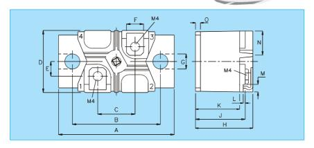
Air distance contact to contact: > 9.2mm
