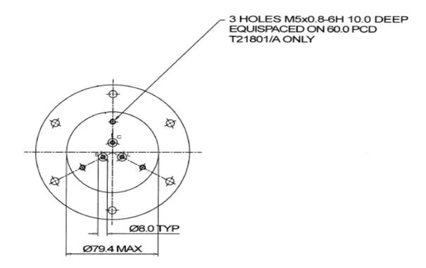
The S71001/A does not have the 3 base holes where as the S71001/AB does, as shown below. The only other difference is the S71001/AB has the C, S, L markings removed and is not polished.
