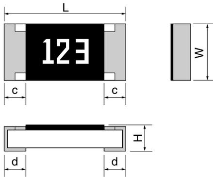
Rated resistance is marked with 3-digit (E24) or 4-digit (E96) on the over coating.
